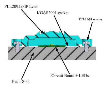
$\label{eq:center} \mbox{ Use TCEI M3 screws}$   $\mbox{ \bullet M3: Maximum tightening torque} \sim 0.4 \mbox{ Nm}$
