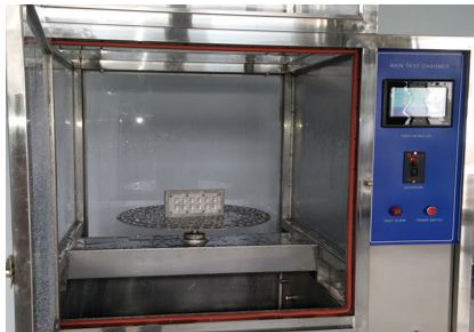
Testing under water jet
