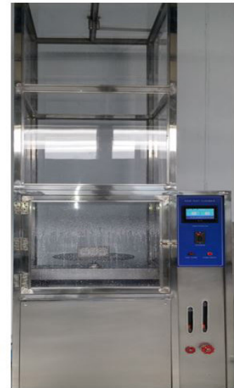
Testing under water jet
