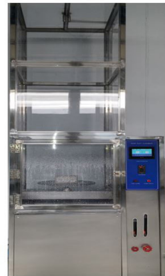
Testing under water jet
