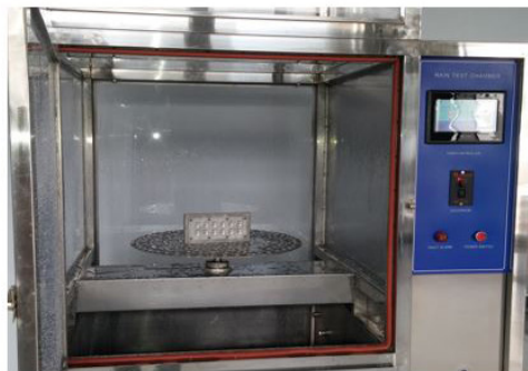
Testing under water jet
