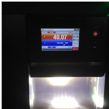
Temperature set in the climatic chamber
