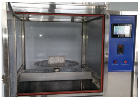
Testing under water jet
