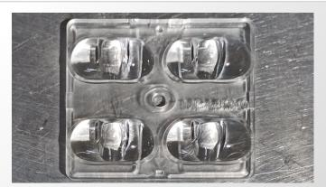
Photo: the part in the climatic chamber after testing.
