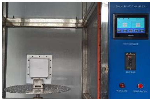
Test Under Water Jet
