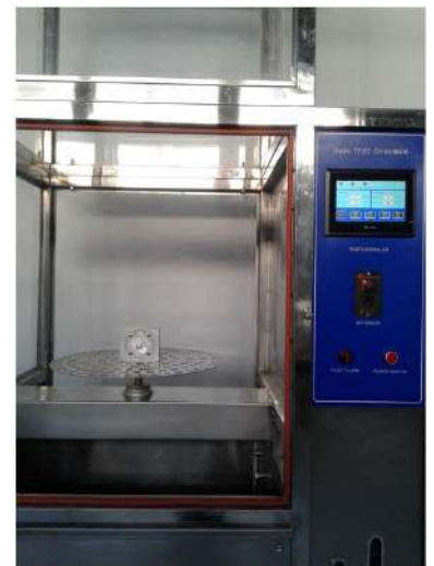
Testing under water jet
