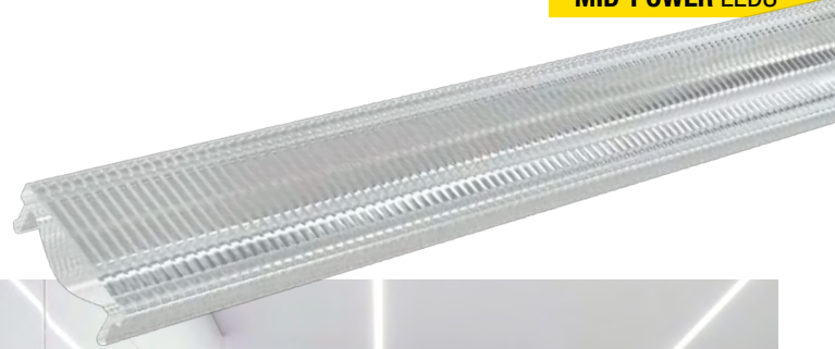
RYO/UW Full angle at 50% from maximum: ~ 90° Full angle at 10% from maximum: ~ 150°
